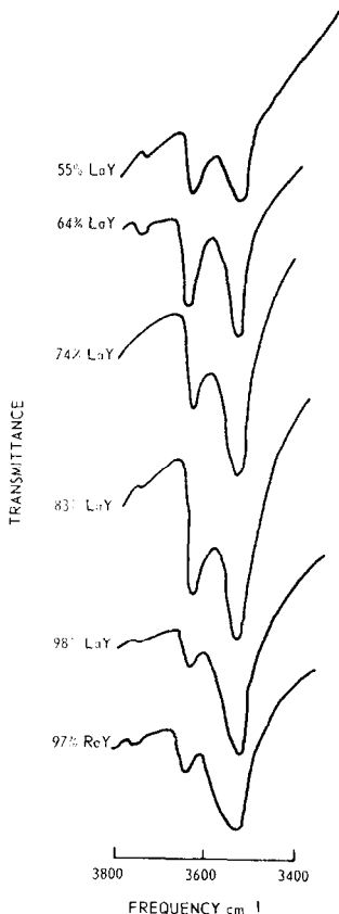
Fig. 2. Infrared spectra of hydroxyl groups on rare-earth exchanged Y zeolite with varying rare-earth contents and after calcination at 400°C.
